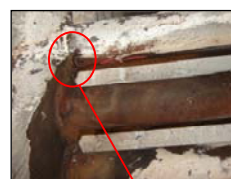
Crack with extension of half perimeter of the tube.
