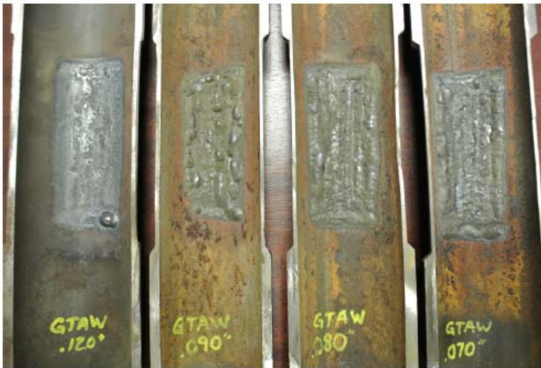
ID: The Melt-thru here is very excessive on the .090", .080" and .070" Samples
