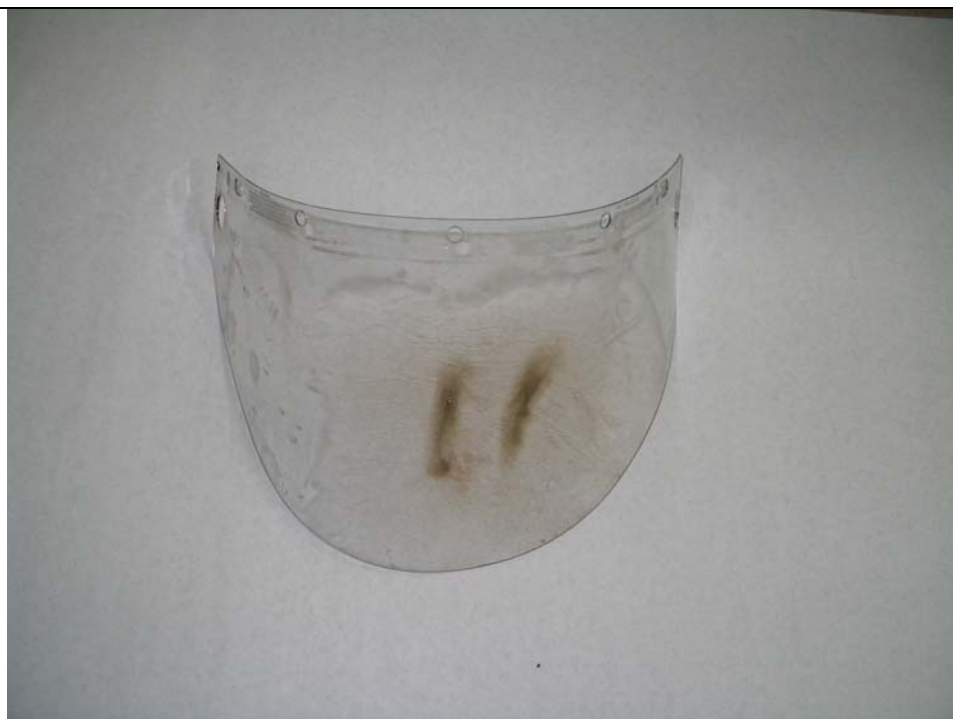
Propionate – After Two Molten Smelt Splashes Note: This shield did NOT burst into flames when splashed with molten smelt
