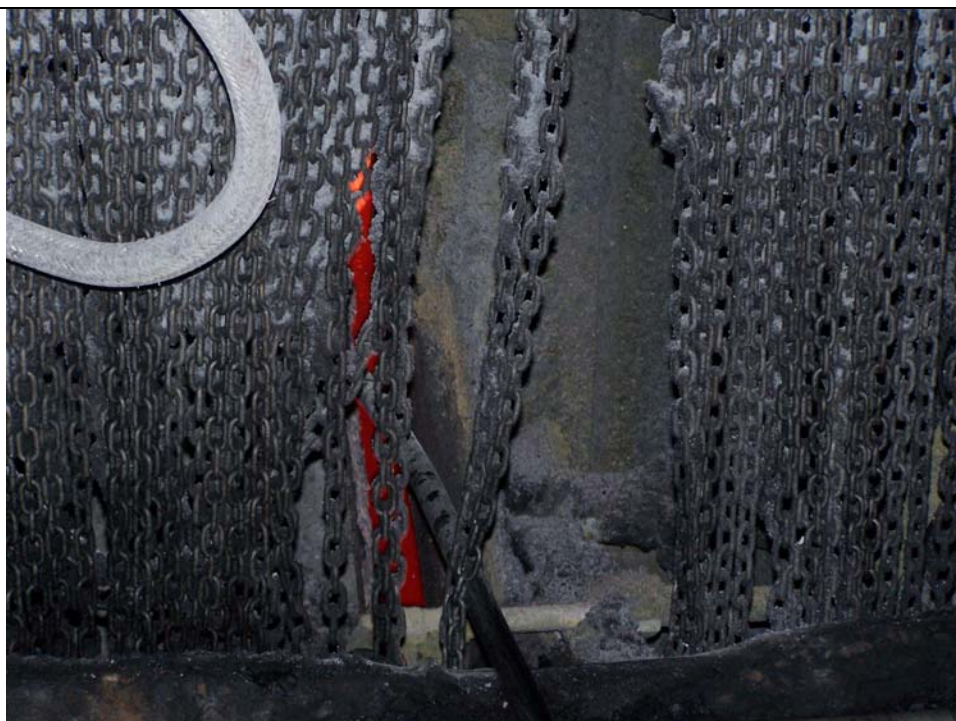
Example "Chain Mail" - Smelt Spout Splatter Protection
