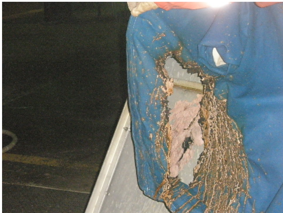
Nomex– After Molten Smelt Splash
