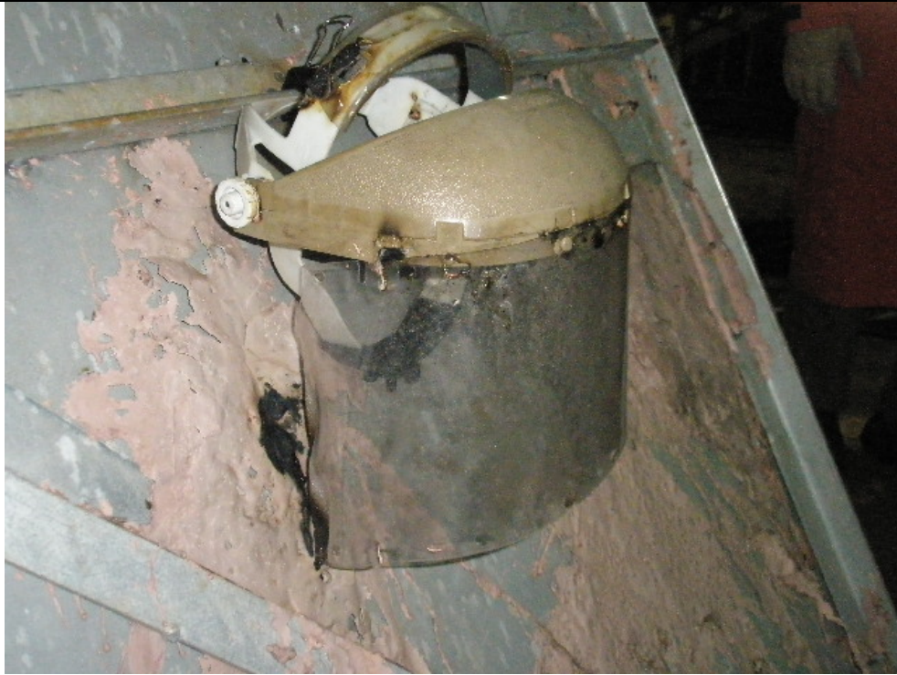
Face Shield Exposed to Molten Smelt
