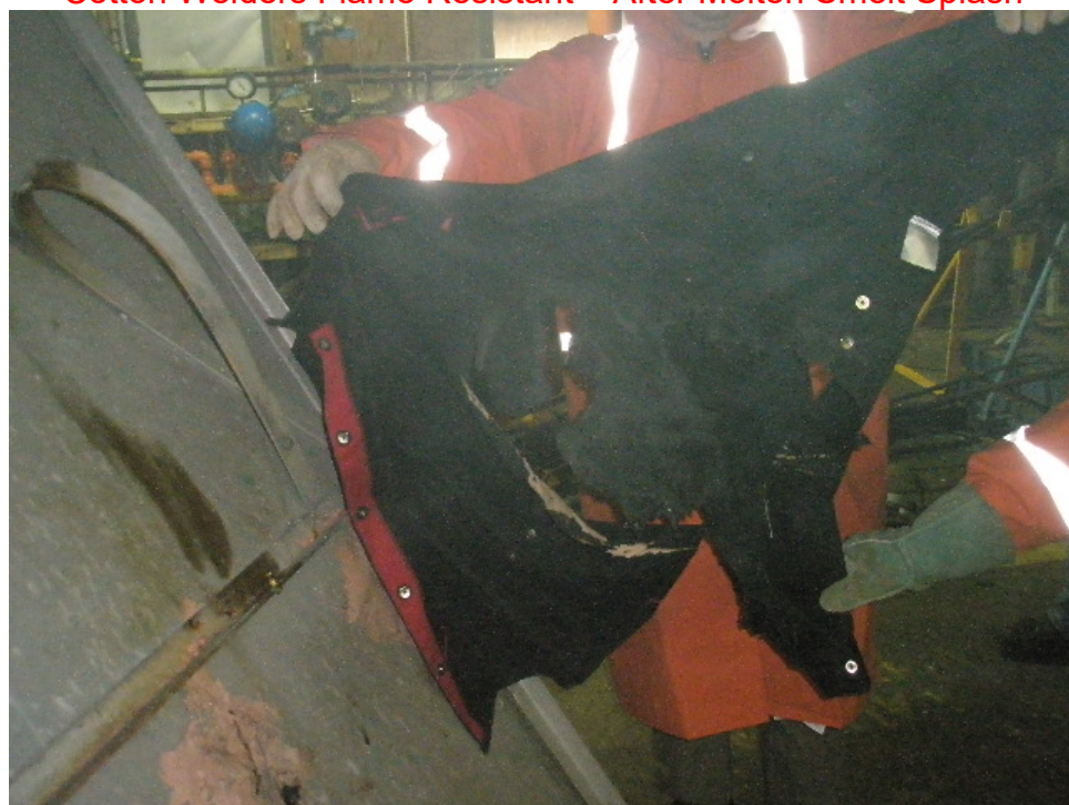
Cotton Welders Flame Resistant – After Molten Smelt Splash - Note Holes
