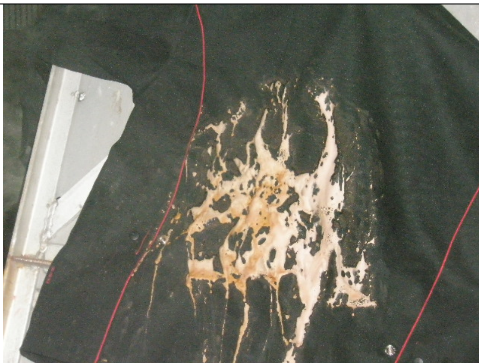
Cotton Welders Flame Resistant – After Molten Smelt Splash
