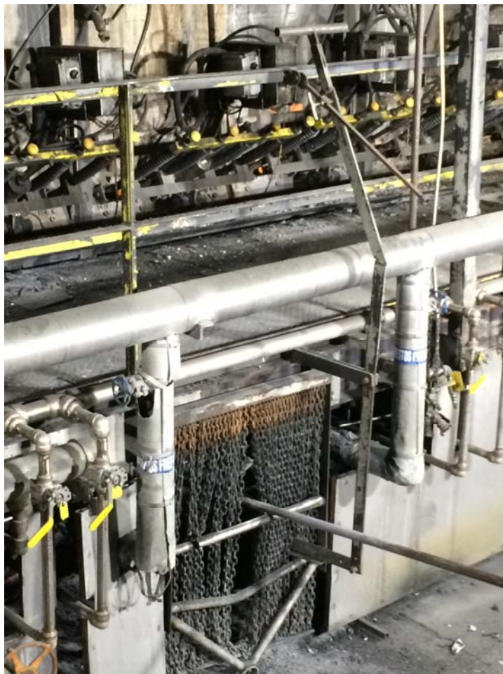
Chain Mail at Smelt Spout with Spout Rod Support
