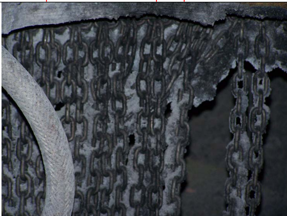
Example "Chain Mail" - Smelt Accumulation on Chains
