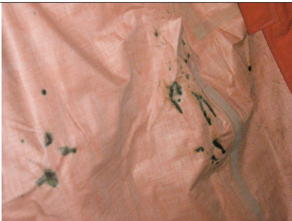
Nomex IIIA / FR Neoprene Jacket – After Molten Smelt Splash
